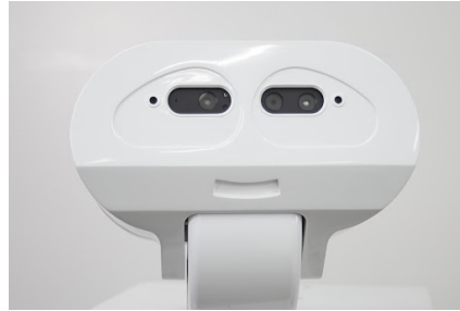
Figure 4: TIAGo++ head with RGB-D camera.
